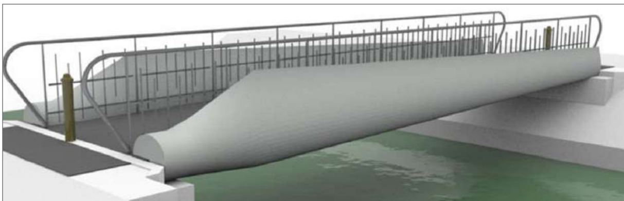
A conceptual design of pedestrian bridge using A29 wind blades as main girders, Re-Wind research project [24]
